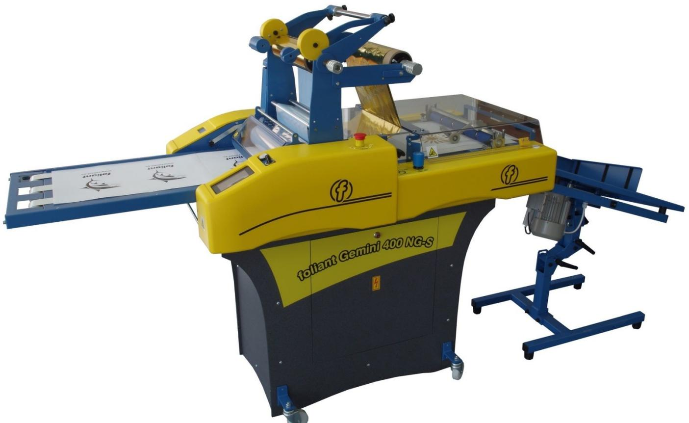
The machine's main feature is a pneumatic pressure system in a heavy duty mechanism enabling to achieve a very high working pressure, one single phase 220 – 240 V supply cable, a small integrated compressor inside the machine frame (i.e. no external source of pressured air is required), a nice design and an easy machine operation.
